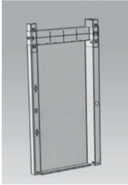
PANEL LATERAL INFERIOR LOWER SIDE PANEL X2
